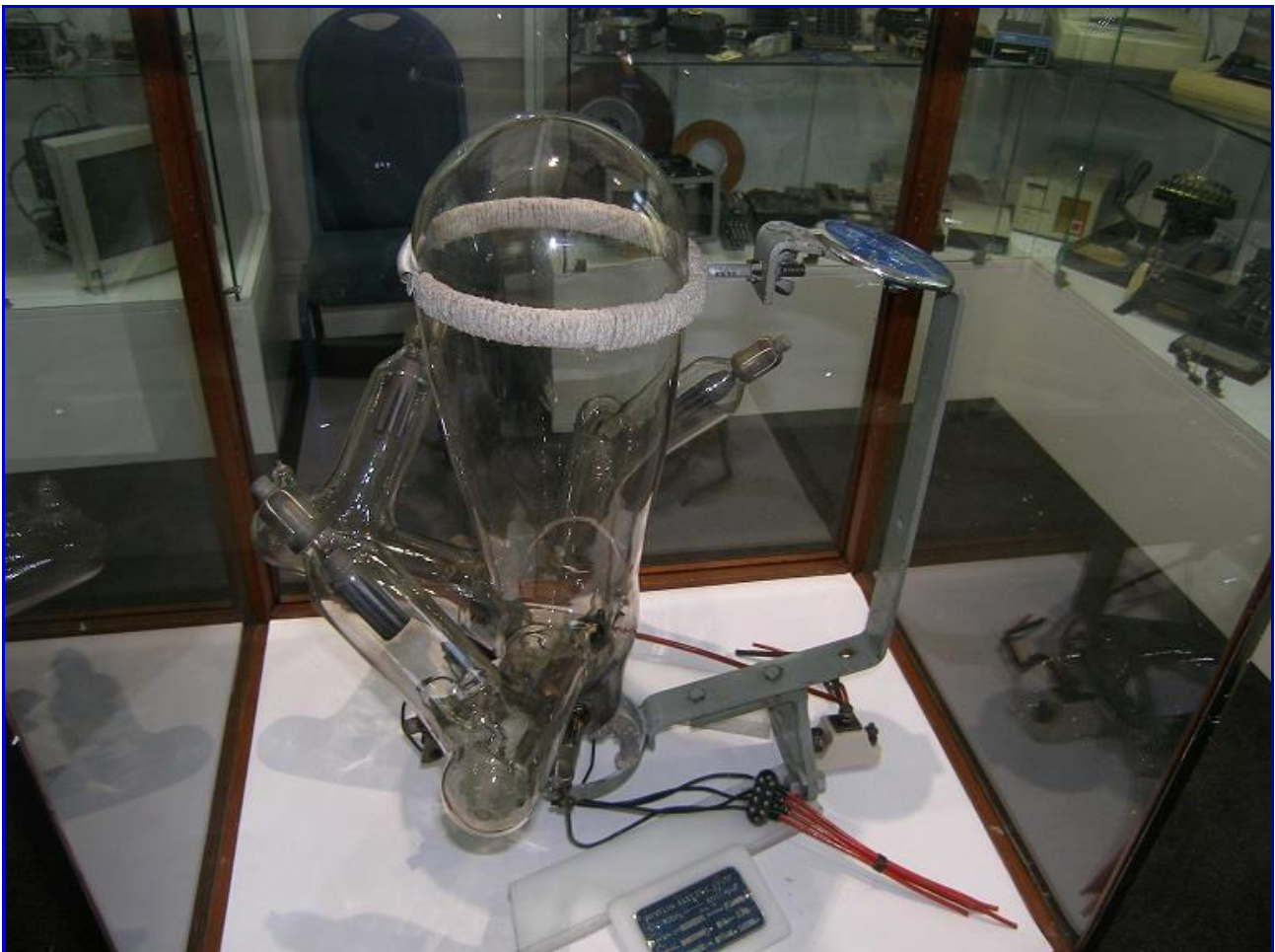
This display is a Nevelin mercury-gas rectifier at the Museum of the South African Institute for Electrical Engineers. This is amongst other numerous magnificent displays, viewed during the AGM of the Antique Wireless Association of South Africa. More on pages 13-16.
